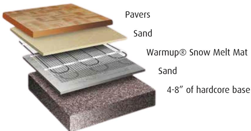
1. Ensure the paving contractor has a solid base of 4"-8" (102-203mm) of crushed rock aggregate tamped down and ready to receive the mortar pour or sand/gravel base.
