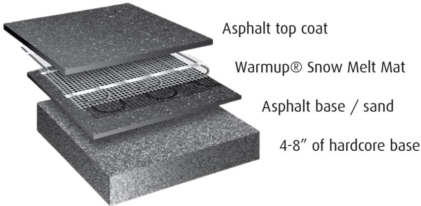
When using the snow melt mats/cables under asphalt, consider embedding them in sand or concrete first.
