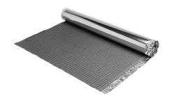
Warmup® Insulated Underlay is a thin insulation barrier that reflects heat upwards, making the underfloor heating system more efficient and effective. It also reduces contact noise. The foil backing acts as an effective moisture barrier.
