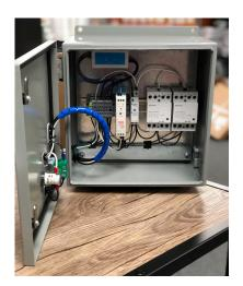
The WSM-252W control panel has two 63A/4-pole contacts that are designed to handle a load of up to 252 amps at 2-phase. At 3-phase, the same control will handle a total capacity of 378 amps. Keeping in mind that 120 sf Warmup snow melting draws 25 amps, this controller could handle up to 1,200 sqft.
