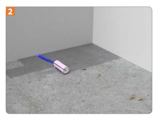
Prime subfloors with a solvent free primer as needed. For proprietary subfloors refer to the manufacturer instructions.
