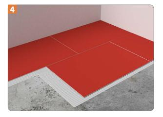
Ultralight should be laid on the freshly applied ribbed bed and thoroughly bedded in to ensure that no voids are left beneath the boards and they are solidly supported. All boards should be laid with staggered joints.
