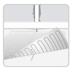
Note: All electrical connections must be performed by a fully qualified and certified electrician. The floor sensor is used for temperature regulation of the floor surface.
