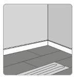
Be careful not to pinch the heating mats when using blocks to hammer the laminate in place. Always keep cardboard or similar handy to place underneath as you move forward in the room. Never make cuts to the planks over the heating system.
