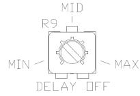
The DEL configuration switch activates the Delay-Off drying cycle timer on the DS- 9C. The timer allows the DS-9C to continue to operate and dry the heated surface through evaporation once precipitation has stopped. The drying cycle reduces the chance of moisture left behind refreezing into ice. This timer is restarted by each sensor trigger. Therefore, the DS-9C will continue to operate as long as it is triggered, then for the Delay-Off period once the trigger clears.
