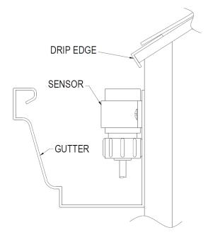
Ten feet of cable is pre-terminated to the sensor head. This cable may be shortened on the controller end as required. Do not add additional cable to the interface. Erratic operation may result. (If the sensor lead needs to be extended, please contact Warmup to order an EX-50.)
