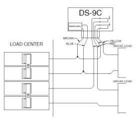
240VAC In, Dual 240VAC Load, Heat Cable or Similar
