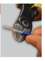
Using the Stanley knife or wire strippers, strip back approximately 7mm of the insulation.
