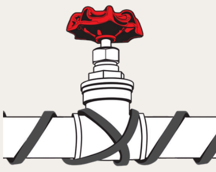
Pipe Trace Cables
