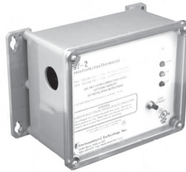
The SST-2 Freeze Protection Thermostat operates from automatically selected operating voltages of 120, 208, 240 or 277 volts, single-phase. They control heater loads of up to 30 amps while consuming less than 2 watts when idling.
