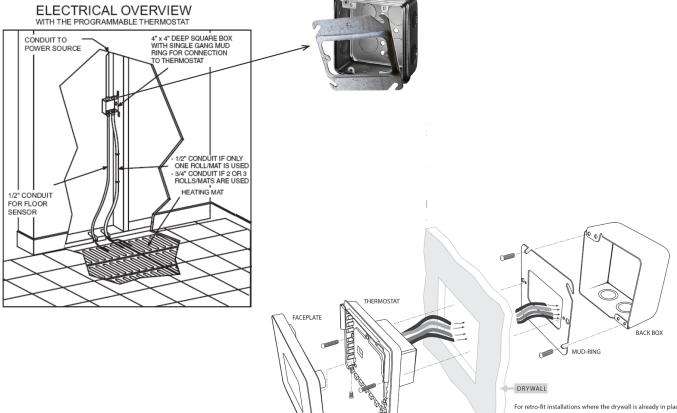
For retro-fit installations where the drywall is already in place, you will need to mud over the mud-ring. In either case, the mud-ring and backbox must be installed behind the drywall.
